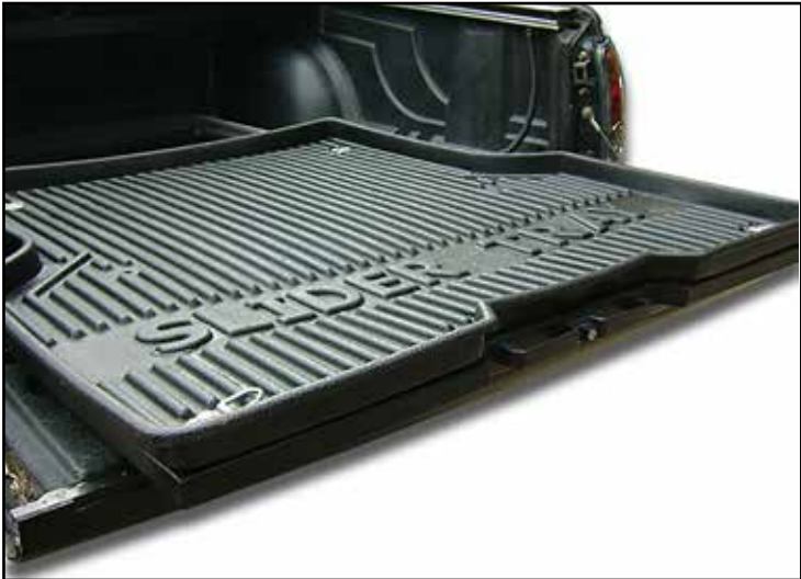
Bed Slide Light Duty -Load rated to 100kg
