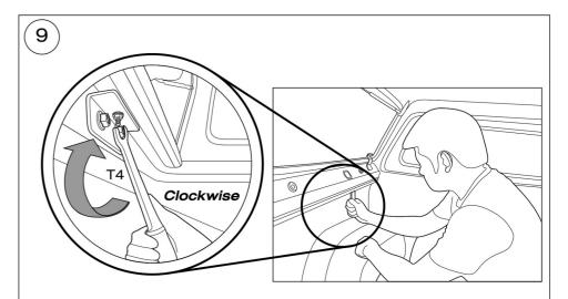
Torque Wrench Tightening To 18-20 Nm
