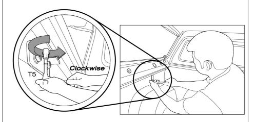
Torque Wrench Tightening To 14-16 Nm
